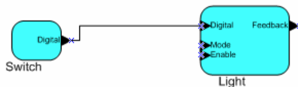
Figure 6. Network Variable Point-to-Point Connection
