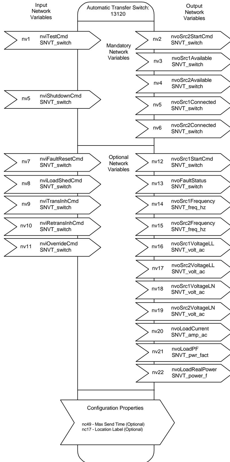
**Figure 1.4** Automatic Transfer Switch Object Details
