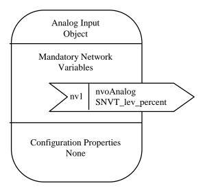
Figure 1.2 Analog Input Object Details
