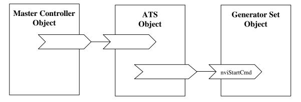
Figure 1.3 Example Usage of Automatic Transfer Switch Object
