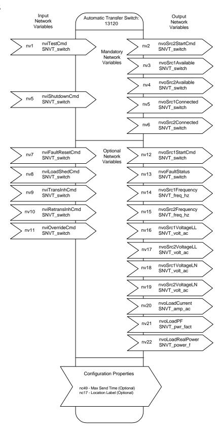
Figure 1.4 Automatic Transfer Switch Object Details
