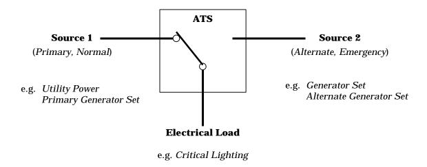
Figure 1.1 Automatic Transfer Switch
