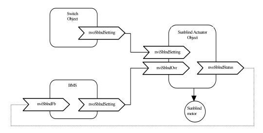
Figure 2 Example Usage of the Functional Block without a Sunblind Controller
