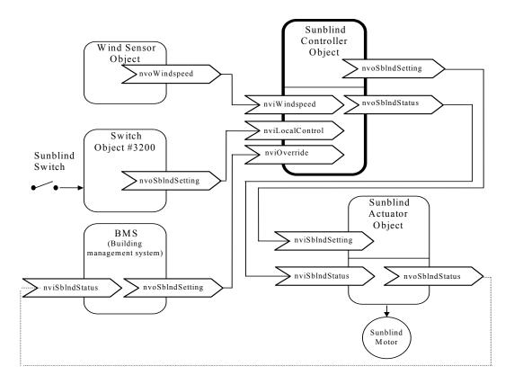
Figure 3 Example Usage of the Functional Block with a Sunblind Controller
