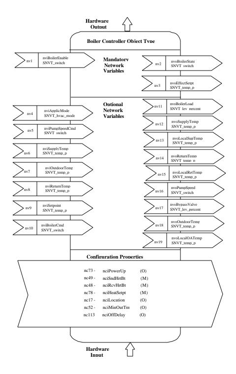
The Boiler controller object can control boiler, heating and pump outputs.
