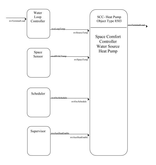
Figure 1.1 WSHP System Drawing
