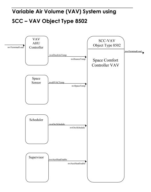
Figure 1.2 VAV System Drawing
