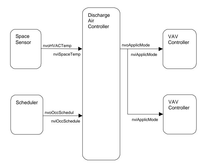
Figure 1 Typical Discharge Air System Drawing
