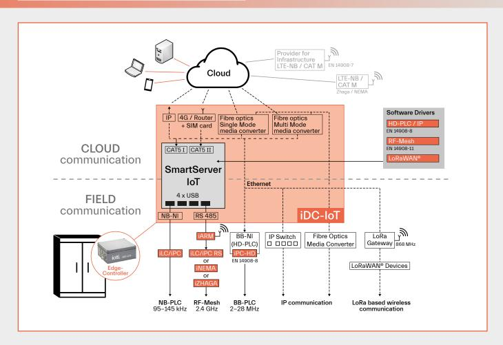
The data concentrator is the intelligent interface between the luminaire controllers in the field and the control technology. With the integrated SmartServer IoT, the iDC-IOT is perfectly suited for the management of all Smart City applications, such as lighting, parking and waste management.
