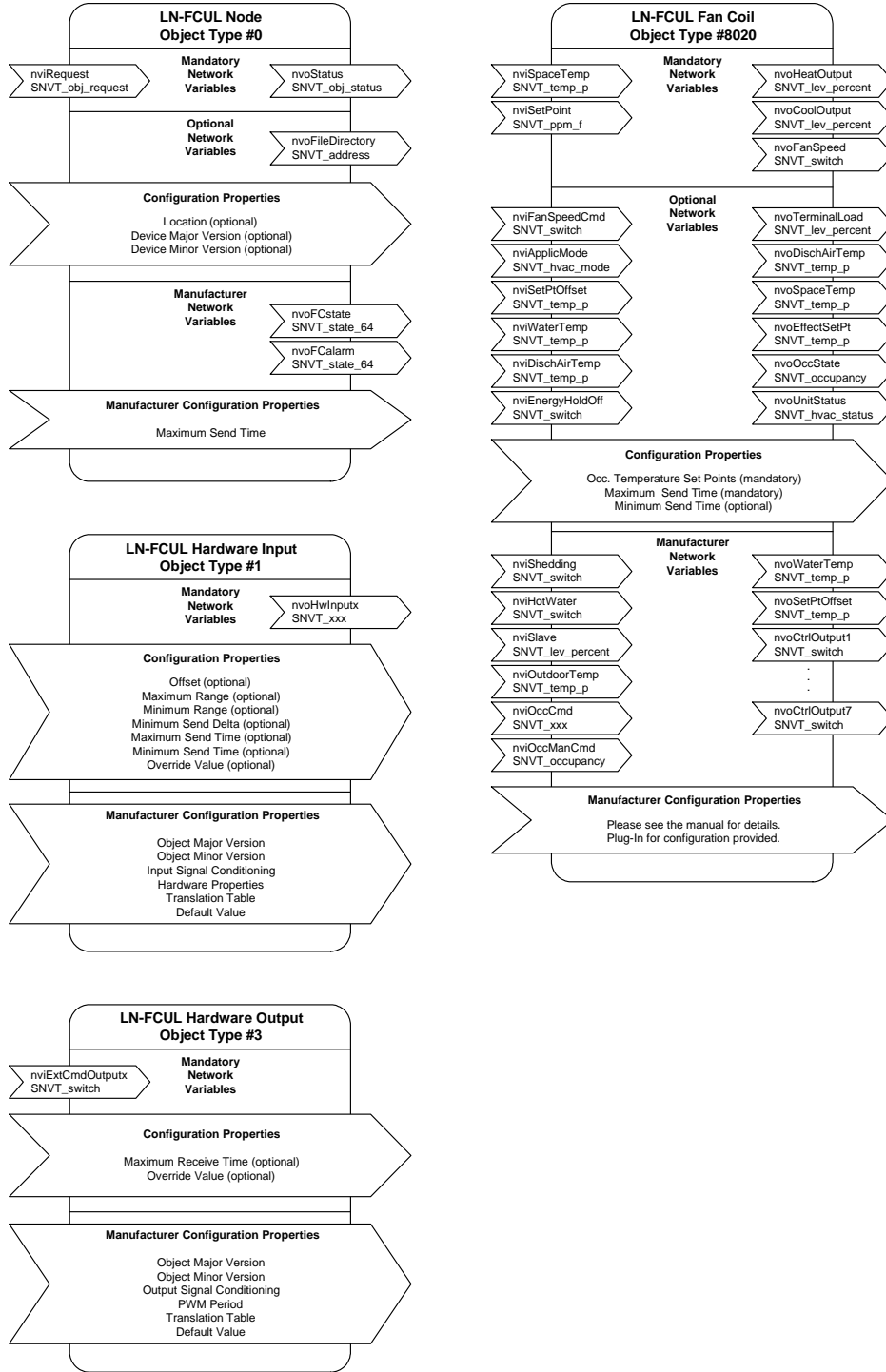
Figure 3: Metasys System LN Series Fan Coil Unit (FCUL) Controller—LONMARK Objects and Network Variables
